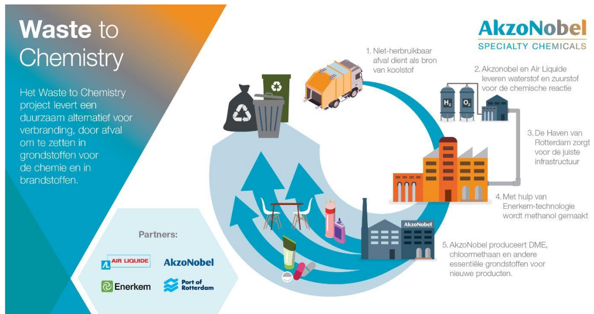
Figuur 9: waste-to-chemistry proces (Akzo-Nobel, 2018)
