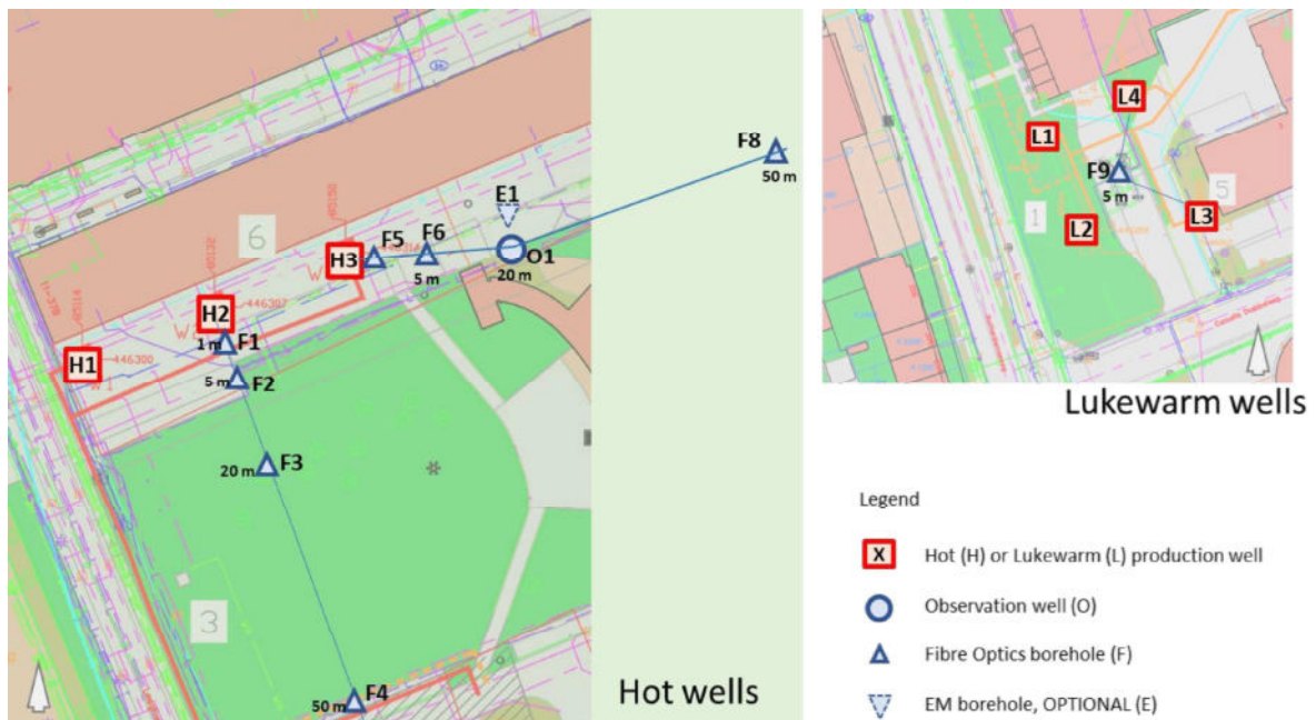
Figure 7. Intended placement of the wells and boreholes
